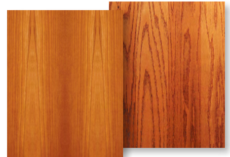
Examples of veneer matching techniques: Book Match (left) and Slip Match (right)
